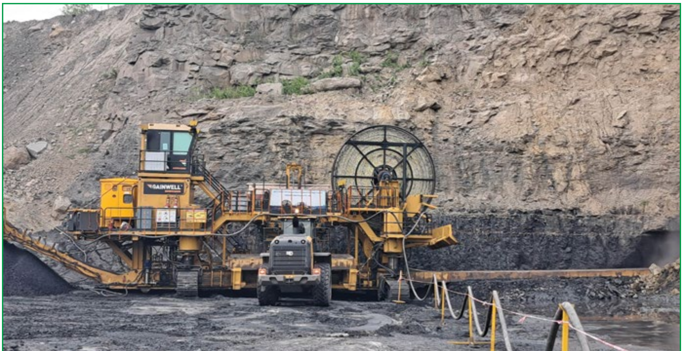
High-wall Mining at Nimcha OC Colliery, Satgram-Sripur Area of ECL
